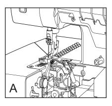
As you sew, you will discover that maneuvering the fabric is different from conventional sewing because the threads form around the stitch fingers. (fig. A)
