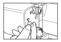
When no trimming is desired, as when stitching on a fold, rotate the cutting blade locking dial clockwise to the LOCK position. The cutting blade no longer moves up and down, but remains in its lowered position. To re-engage the cutting blade, turn the cutting blade locking dial half of a turn counter-clockwise. The blade will start moving automatically when you start serging.
