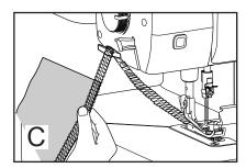
With the needle and looper threads under the foot and to the back, lower the presser foot. While holding the threads in your left hand, press down on the foot control gently to begin a thread chain before serging fabric. (fig. A)
