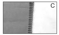
Set up the machine for 2-thread flatlock-wide but the needle threading path is different for this technique.
