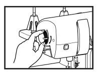
The presser foot pressure has been preset at the factory and rarely needs adjustment. You may find it necessary, however, to decrease the pressure for thick fabrics or increase pressure for thin fabrics to feed more smoothly under the foot. Turn the presser foot pressure adjustment dial on left side of the machine.
