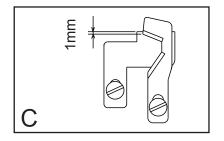
The lower fixed blade is made of a special long lasting steel and does not require frequent replacement.
