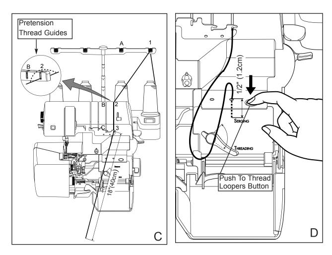
\*Be sure at least 1/2" of thread is inserted into the threading port.
