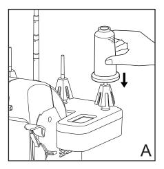
When using threads on cones or king spools place the cone or spool securely over the cone holders furnished on your machine. To avoid bending the thread stand, you may need to place one hand under the stand while positioning the cone. The cone holders prevent the cone or spool from spinning, enabling the thread to feed evenly. (fig. A)
