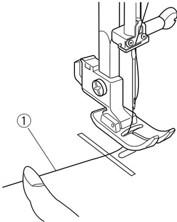
1 With the presser foot in the raised position, hold the needle thread lightly with your left hand.
