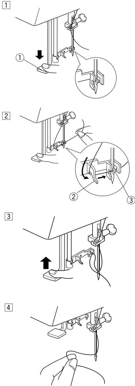
1 Raise the needle to its highest position and lower the presser foot. Push down the needle threader knob as far as it will go.
