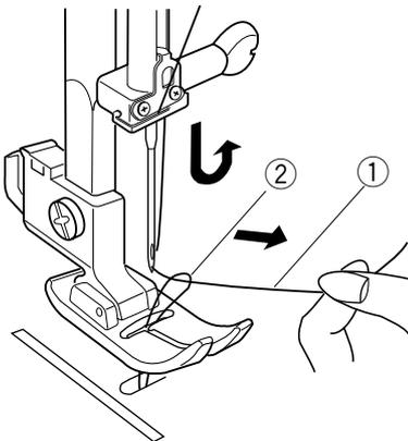
2 Turn the handwheel slowly toward you one complete turn. Bring the bobbin thread up by pulling the needle thread as illustrated.
