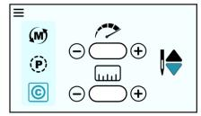
The needle cycles continuously, but it changes speeds to maintain the stitch length when the machine is moved.
