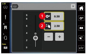
1 Permanent Alteration of Thread Tension
