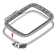
> Place the template (1) in the inner hoop, so that the bernette logo is aligned with the arrow marking at the front edge so that it clicks into place.
