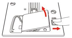
> Insert a new bobbin so that the thread is wound anti-clockwise.
