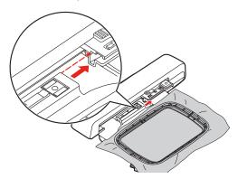
> To remove the hoop, press the securing lever and pull the hoop backwards.
