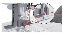
> To cut off excess thread, take the thread end and carefully pull it over the thread cutter. **Please Note:** Use the right thread cutter only when threading.
