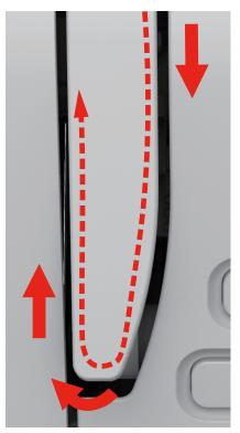
> Guide the thread at the top from rigth to the left through the thread take-up lever and then down again.
