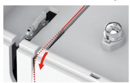
> Guide the htread downwards around the thread take-up lever cover.
