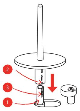
**Inserting Thread Spool**
