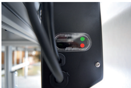
Fig. 2: LEDs on the drive motors
