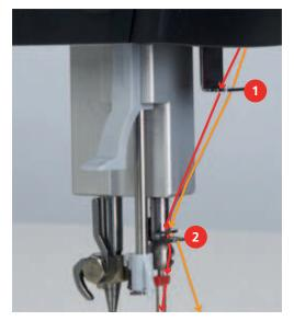
> Place the thread into the slot of the manual threader.
