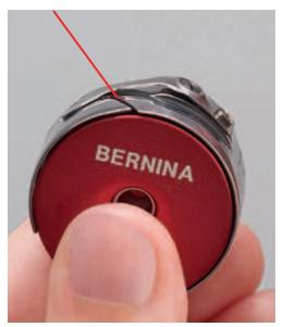
> Pull the thread to the left under the spring and into the opening at the end of the spring.
