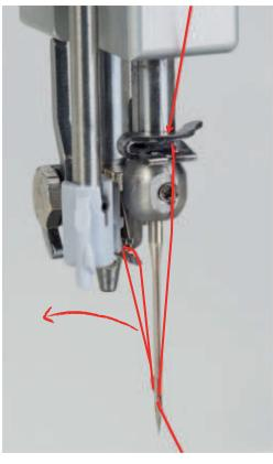
> Pull the thread over the thread cutter (13) from the back to the front, then cut.
