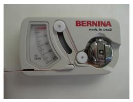
> Pull on the thread steadily and read the thread tension.
