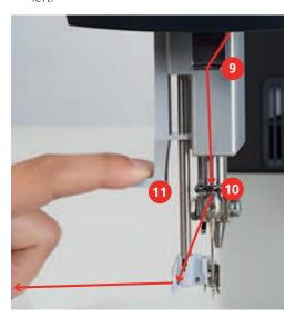
> Pull the thread from left to right in front of the hook (12) and the needle and through the thread guide until it catches on the wire hook.
