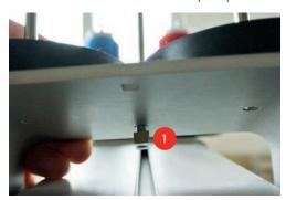
> Place the spool holder on the machine such that both spool pins (1) are positioned in front of the thread guide (2).
