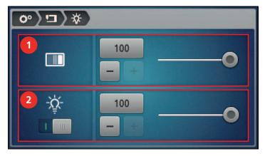
> Switch the sewing light on or off and adjust the brightness in the bottom section of the screen (2).
