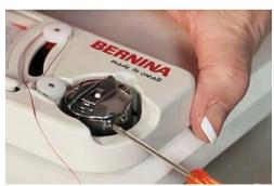
> Hold down overhanging thread with your finger and cut with the thread cutter.
