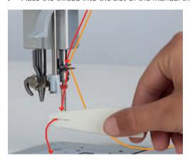
> Thread it into the right needle using the needle threader.
