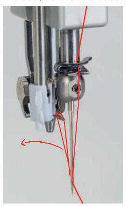
$>\;\;$  Pull the thread over the thread cutter (13) from the back to the front, then cut.
