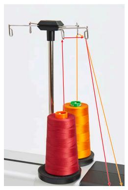
> First, guide the thread on the left-hand side of the machine through the upper right thread guide, then pull in the direction of the arrow through the lower thread guide.
