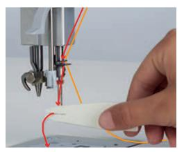
> Thread it into the right needle using the needle threader.
