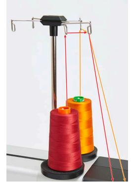
> First, guide the thread on the left-hand side of the machine through the upper right thread guide, then pull in the direction of the arrow through the lower thread guide.
