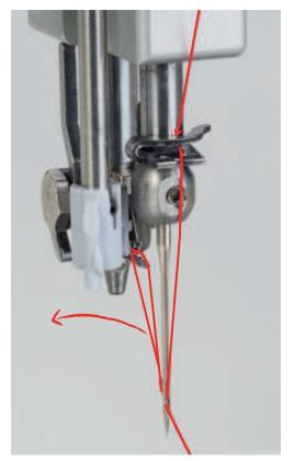
> Pull the thread over the thread cutter (13) from the back to the front, then cut.
