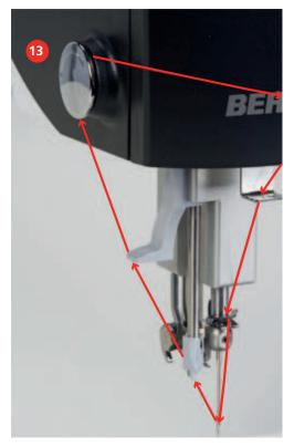
Check whether the thread is correctly positioned in the thread tension unit.
