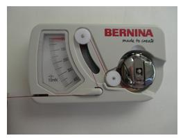
> Pull on the thread steadily and read the thread tension.
